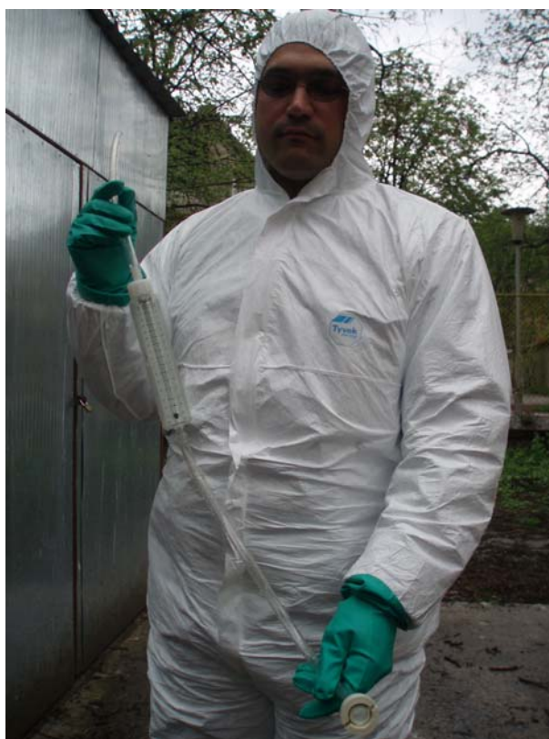
Flow-metre for simple and quick test of the yield of sprayer nozzles
